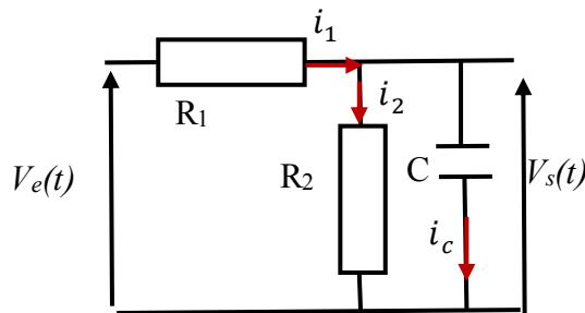
$$v_e(t) = R_1 i_1(t) + v_s(t) \quad (1)$$
