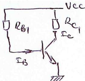
$$* V_{CE} + R_c I_c = V_{CC} \Rightarrow R_c = \frac{V_{CC} - V_{CE}}{I_c}$$
