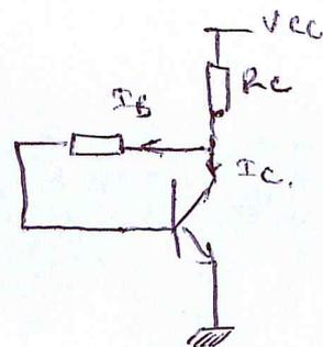
au point de repos :  $R_c = \frac{V_{CC}}{2 I_{C_0}} = \frac{10}{2} = 5k\Omega$
