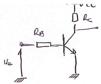
droite de charge:  $V_{CE} + R_C I_C = V_{CC} \Rightarrow I_C = \frac{V_{CC} - V_{CE}}{R_C}$
