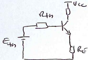
$$R_{th} = \frac{R_{B1} R_{B2}}{R_{B1} + R_{B2}}, \quad E_{th} = \frac{R_{B2}}{R_{B2} + R_{B1}} V_{CC}$$
