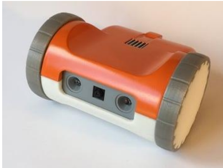
Fig 4.6 FPV Robot Controlled by RPI Zero W
