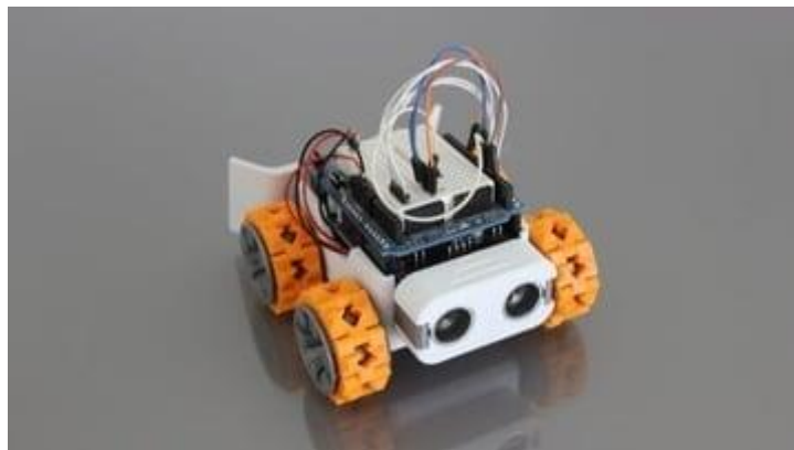
Fig 4.3 Project Robot based on Raspberry Pi Pico
