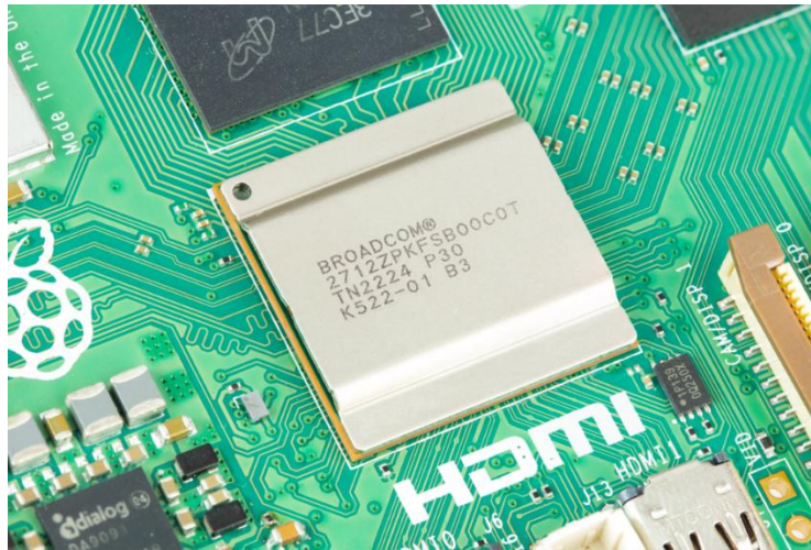
Figure 3 : the main SoC on RPI-5, Broadcom 2712
