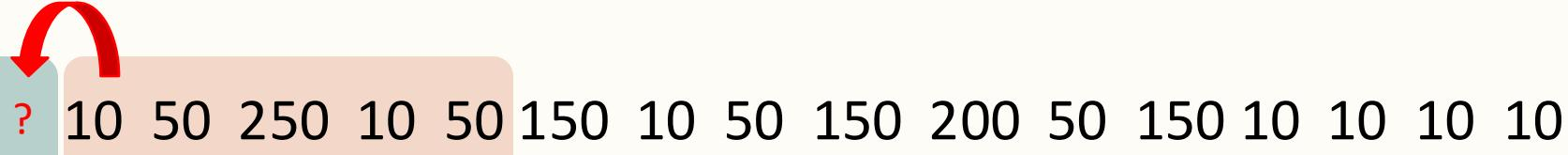
Diagram illustrating the LZSS encoding of a sequence of bytes. The sequence is: 10 50 250 10 50 150 10 50 150 200 50 150 10 10 10 10. A red question mark is placed in the first byte position, and a red curved arrow points from the question mark to the second byte position (50).
