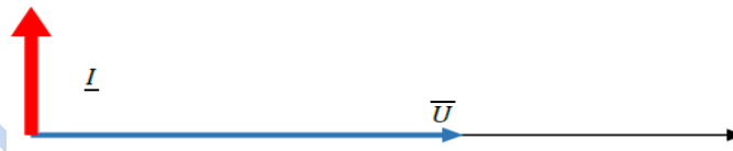
Fig. 2.22 Capacitor ;voltage and current vectors
