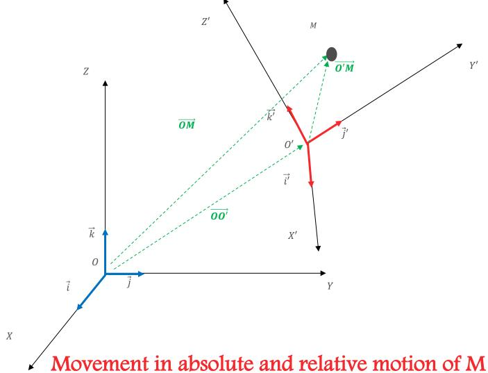
Absolute Motion of M R(o,x,y,z)(Fixe) R'(o',x',y',z') Relative Motion of M
