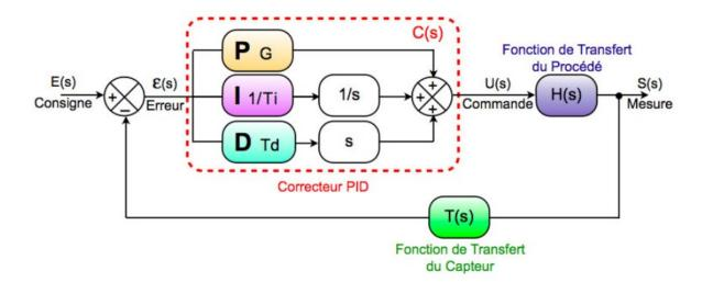
The role of the regulator is to limit the variations of the measured quantity when the system is subjected to disturbances of the quantities
