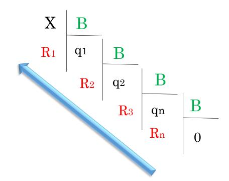
$$(X)_{10} = (R_n..R_3R_2R_1)_{\mathbf{B}}$$
