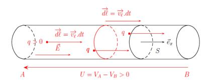
During the elementary time interval dt, the quantity of electricity dq that passes through a surface S in the positive direction, denoted by ex is the chargecontained in the cylinder with generator dl and base S.
