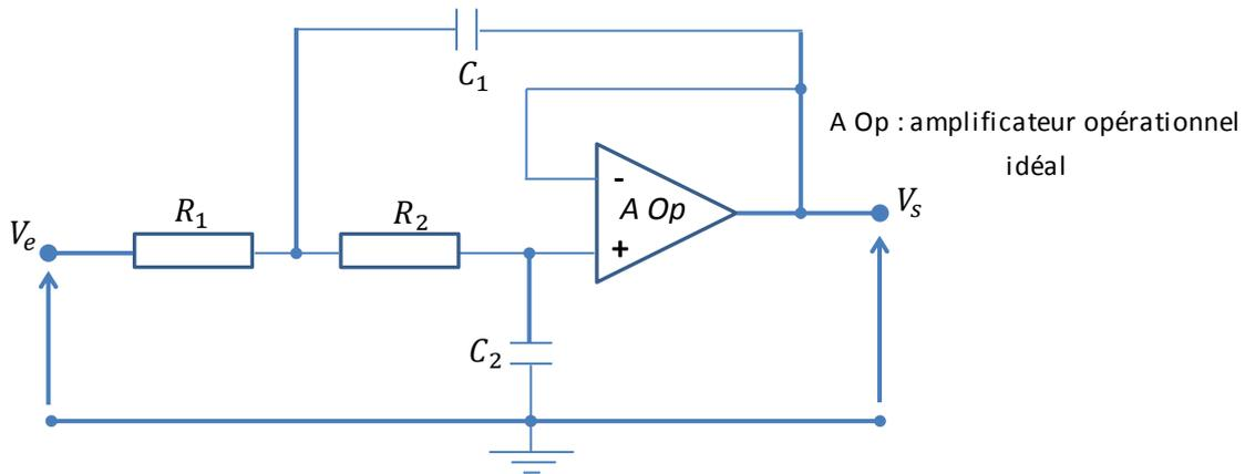
$$H(p) = \frac{w_0^2}{p^2 + \frac{(R_1 + R_2)}{C_1 R_1 R_2} p + w_0^2} \quad \text{avec} \quad w_0^2 = \frac{1}{R_1 R_2 C_1 C_2}$$
