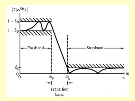
• As indicated in the figure, in the passband, defined by  $0 \le \omega \le \omega_p$ , we require that  $G(e^{j\omega}) \cong 1$  with an error  $\pm \delta_p$ , i.e.,
