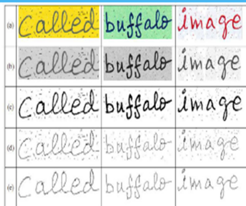
Fig.2. Word Image Pre-Processing (a) Input Scanned Word Images; (b) Word Images after Gray Scale Intensity Threshold; (c) Word Images in Binary Format; (d) Word Images after Thinning; (e) Word Images after Noise Removal.
