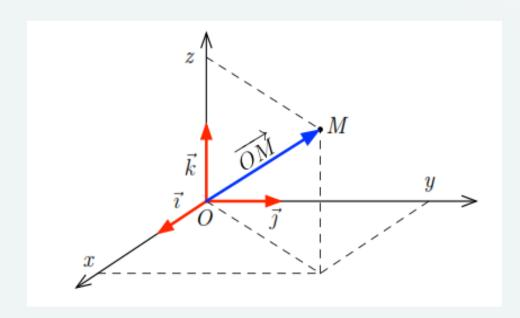
• The cartesian coordinates of a point M are (x,y,z) The vector  $\overrightarrow{OM}$  wish relie between the origin point and point M is writen as:
