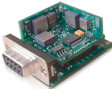
FIGURE 4.8 – Centrale inertielle Crista de Cloud Cap Technology.
